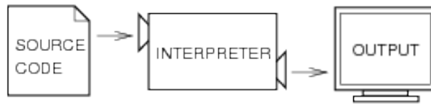
Figure 1.1: An interpreter processes the program a little at a time, alternately reading lines and performing computations.
